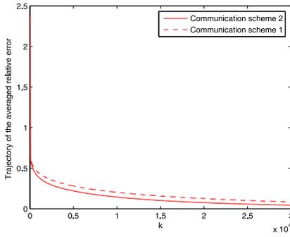
Fig. 3. Trajectories of the averaged relative errors under the communication schemes 1 and 2.
