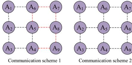
Fig. 1. Two communication schemes. In Communication Scheme 1, only the links represented by the black lines are active at odd time instants and only the links represented by the red lines are active at even time instants, i.e.,  $h = 2$ . In Communication Scheme 2, all these links are active at each time instant.
