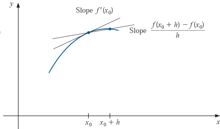
$$\begin{aligned} f'(x_0) &= \frac{1}{h} (f(x_1) - f(x_0)) - \frac{h}{2} f''(\xi_0) \\ f'(x_1) &= \frac{1}{h} (f(x_1) - f(x_0)) + \frac{h}{2} f''(\xi_1) \end{aligned}$$
